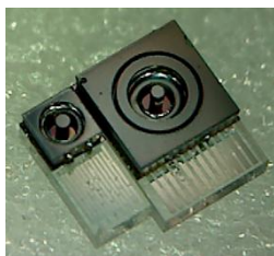
Fig.1 – 3D force sensors developed at MFA MEMS laboratory
