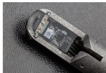
Fig.2 – surgery gripper with implanted force sensors
